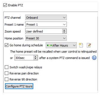
PTZ channels can be added in two ways: by selecting Onboard or a Serial Port.
