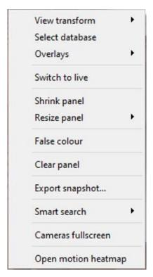
**View transform:** allows transforming images for cameras with special lenses. (For example, 360-degree cameras.)
