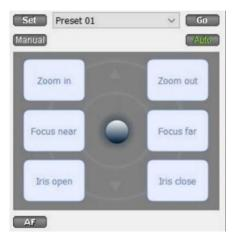
With a Pan-Tilt-Zoom (PTZ) camera, an operator can manipulate the camera's direction, Zoom, focal distance (Focus) and amount of light (Iris).
